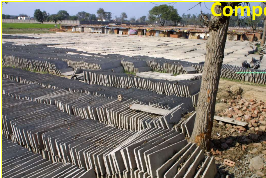
Semi-mechanized Production of Precast Building
