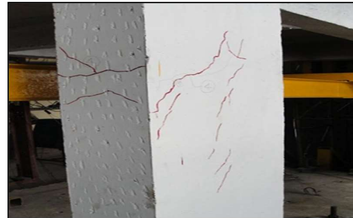
Cracks on mid-span of column at higher drift
