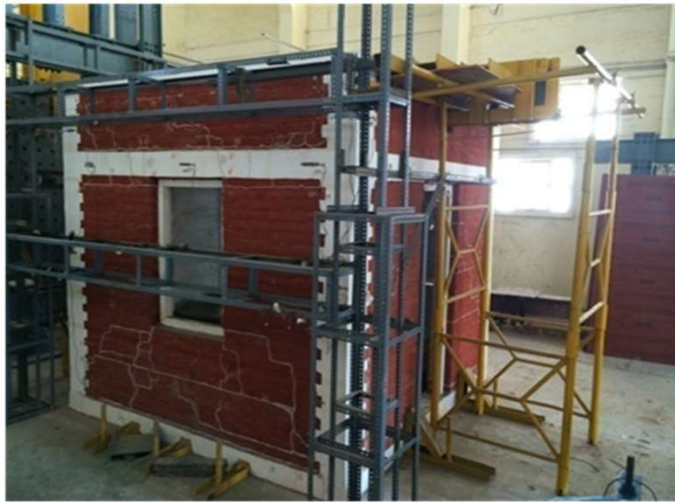
Cracks in CM building Model
